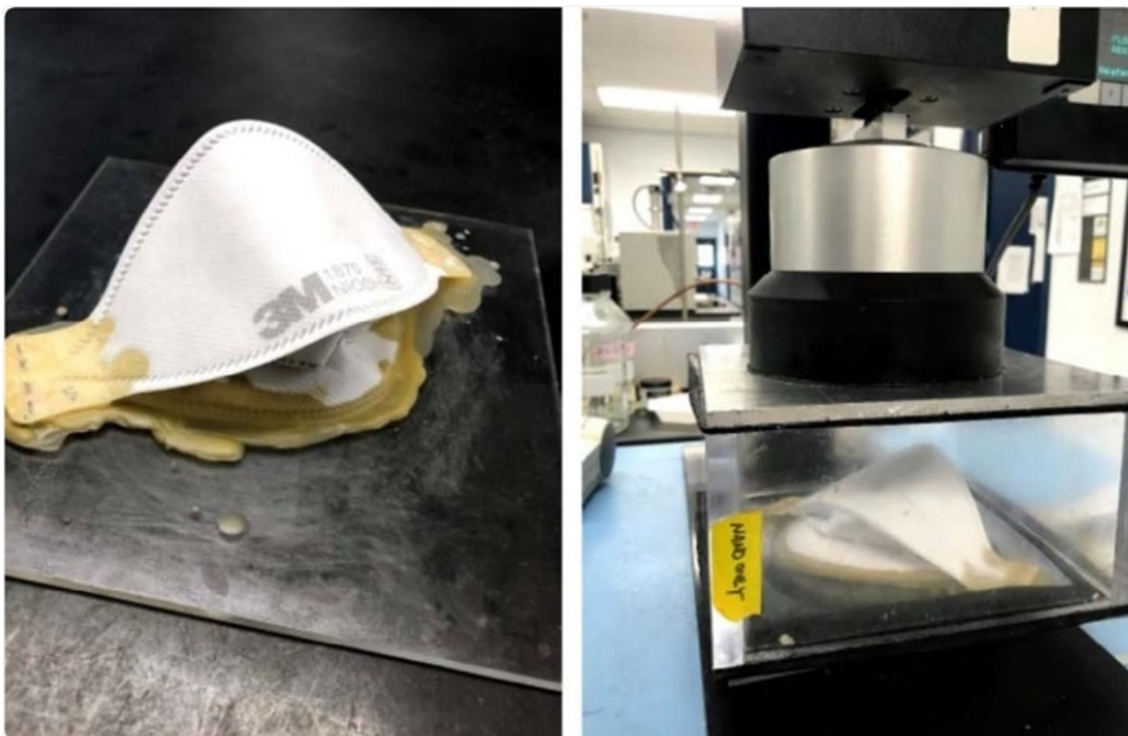
Image of N95 respirator after ten treatments with 450 ppm ozone for 2 hours at 75-90% humidity. There is little noticeable wear on the respirator after extended exposure to ozone.
